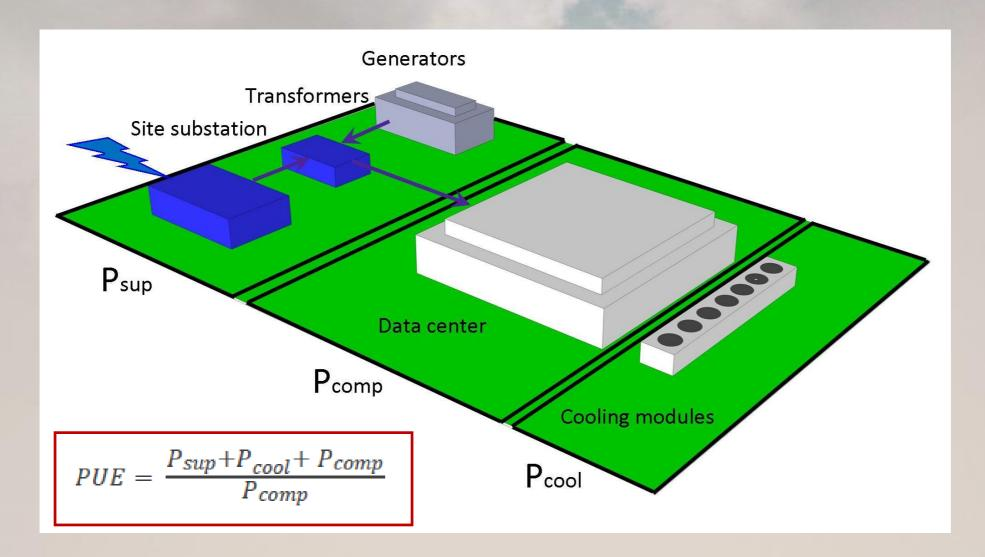
Improving power distribution and cooling improves PUE, but has no impact on amount of power used for computation
